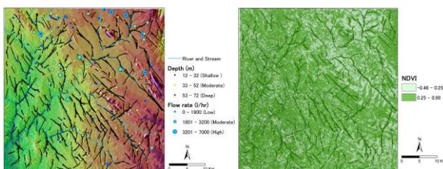
Fig. 3. Grouped lineaments overlaid by water borehole data (left) and by NDVI (right).
