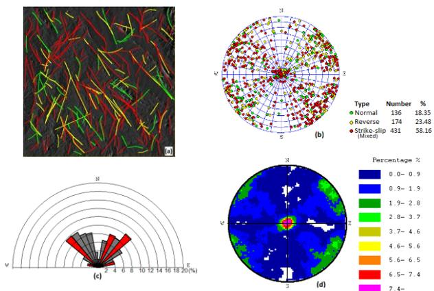
Fig. 2. (a) Shaded relief map overlaid by modeled faults, (b) fault type frequency, (c) rose diagram showing strike of the lineaments and (d) Schmidt net.
