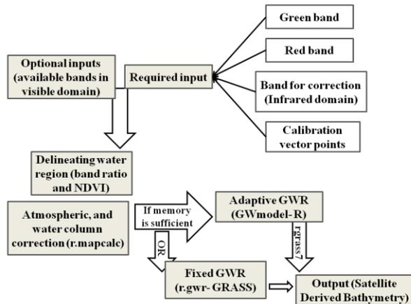
Figure 1. Flowchart of workflow of i.image.bathymetry.
