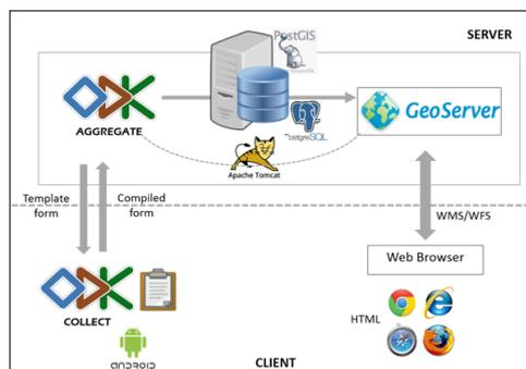
Figure 1: System architecture
