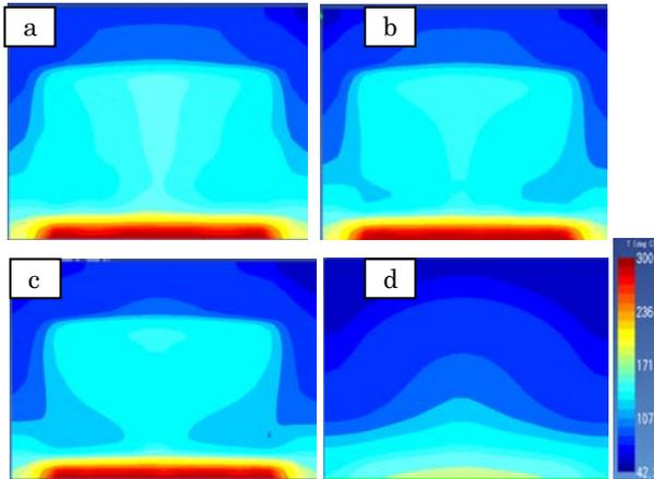
Fig. 2: Temperature distribution development result after 10,000 years simulation time. a = sliced in the middle part of the model ( $x = y = 2000$  meter), b = at 2500 meter, c = at 3000 meter, d = at 4000 meter (boundary).
