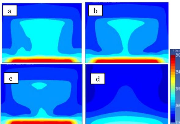
Fig. 3: Temperature distribution development result after 20,000 years simulation time. a = sliced in the middle part of the model ( $x = y = 2000$  meter), b = at 2500 meter, c = at 3000 meter, d = at 4000 meter (boundary).
