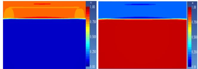
Fig. 4: Vapor (left) and liquid (right) reservoir development after 10,000 years simulation time.
