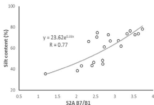
Figure. 2 Cross-relationship of *in-situ* silt content with simulated S2A ratio band reflectance.
