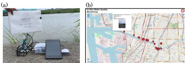
Figure 4: (a) Sample collections and measuring method (b) Data collection points displayed on Web interface-GIS Client
