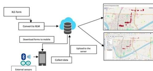
Figure 2: Data flow of developed system
