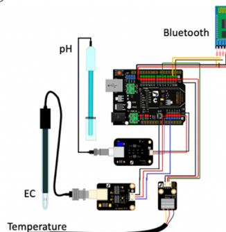
Figure 1: Schematic diagram of system components
