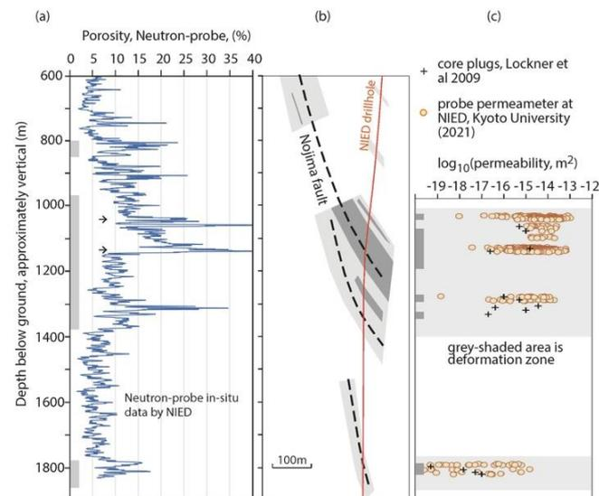
Figure 2. Example of fault zone properties at NIED drill hole, Hirabayashi drill site, Awaji Island. (a) Neutron-probe in-situ porosity, NIED data, and (b) drill core rock matrix permeability tested by Kyoto University.
